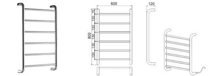
CE 認證 Model: HTR 800x600/6 Material:Stainless steel 不銹鋼 Heated towel rails 暗裝式/明裝式暖毛巾杆(圓) Bars:6 Size: 800Hx600W Power: 50W Size: 800x120x600mm 尺寸: 600x120x600mm
